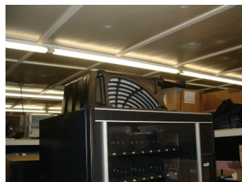
INSTALL FILTER IN FILTER COVER AND SNAP INTO POSITION
