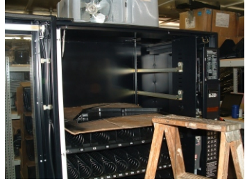
REMOVE UPPER TRAYS TO ACCESS TOP OF MACHINE *
