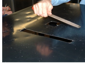
CUT INLET AND OUTLET AIR HOLES
